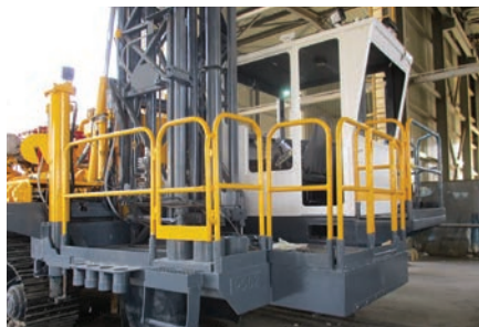
Rebuilds will incorporate extended decks and walkways to allow better access to components for both operations and maintenance crews.
