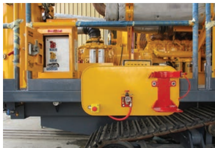
The emergency panel and isolation panel are mounted next to each other to improve rig safety.
